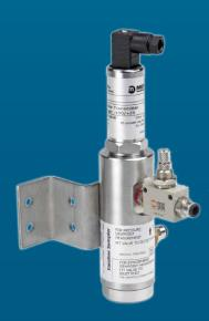
97076 Issue 08 May 2013 The Easidew Sampler is a modular low-cost, self-contained, filtration block and flow control arrangement which is suitable for any Michell impedance dew-point transmitter with 5/8" - 18 UNF process connection size, and is able to perform dew-point measurements at atmospheric (1 barg (14.5 psig)) or system pressures (10 barg (145 psig)).
